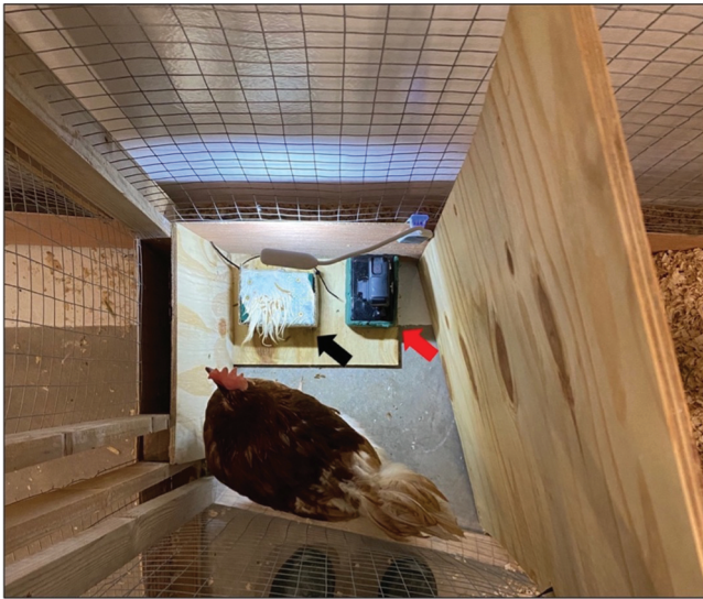
Figure 2. Set up of the test pen used for the study. The black arrow indicates the chicken model (foam block covered with feathered chicken skin). The red arrow indicates the high-speed video camera.
