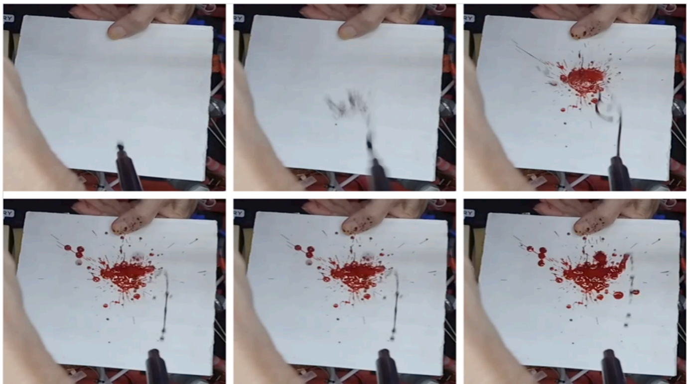
Fig. 3. 3a (top-left), 3b (top-middle), 3c (top-right), 3d (bottom-left), 3e (bottom-middle), 3f (bottom-right). Fluid volume ejection and stain creation in microgravity.
