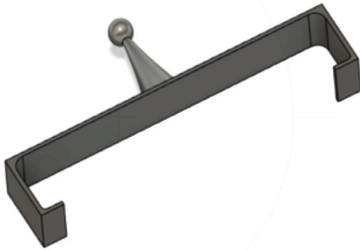
Fig. 2. Smartphone add-on for vibration testing.
