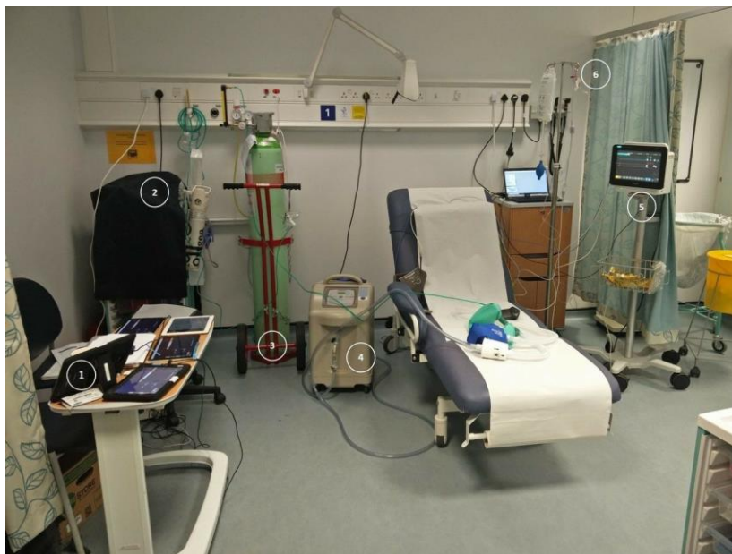
Figure 9 – Hypoxia study day set-up. Legend: 1: tablets linked with AMD devices (4 Samsung TAB A, each linked with one AMD: AP-20, WristOX2 3150 BLE, CheckMe™ O2 and VitalPatch®. 1 iPad four connected to the wavelet). 2: resuscitation trolley and oxygen. 3: 3%–7% oxygen in nitrogen cylinder. 4: hypoxicator apparatus. 5: Philips monitor (model MX450) connected to laptop (IX trend software). 6: drip stand with the arterial line pressure bag. Extracted from the original protocol (CC BY 4.0) (Areia, Carlos et al. 2020a).
