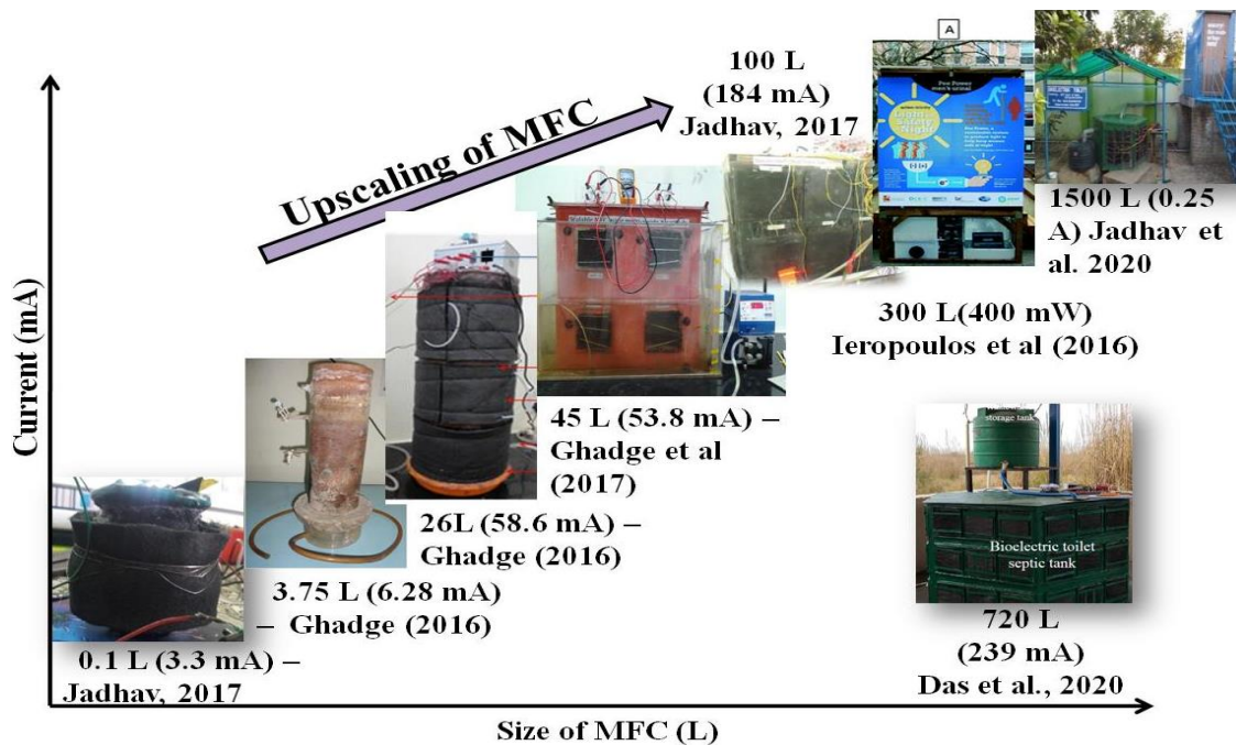
Figure 6: Development of lab-scale to scaling-up ceramic membrane based MFCs along with current generation
