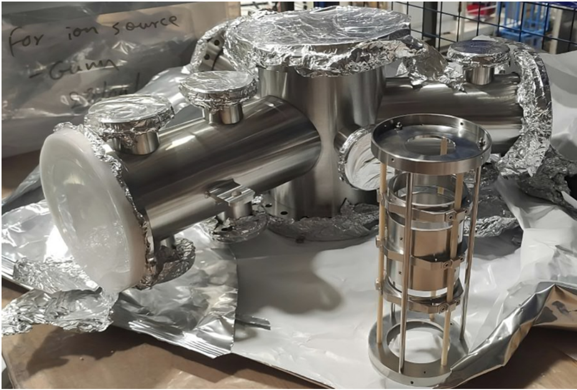
Figure 5.31: The “Starship” deflection chamber together with one of the inner ion lens assemblies (private photo gallery).
