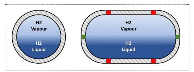
**Figure 1.** Front and side views of conceptual LH2 storage tanks. Liquid and vapour Hydrogen, inner shell, insulation, and outer shell shown. Indicative peripheral or axisymmetric positions of potential inner-outer shell thermomechanical supports shown on the side view
