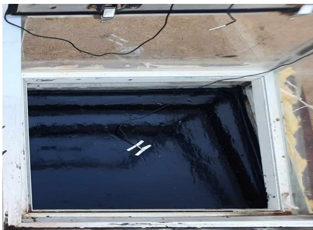
Figure.3 conventional solar still with nano coating.
