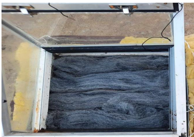
Figure.4 conventional solar still with nano coating and heat transfer medium.
