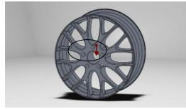
Figure 8. Gravity load point.
