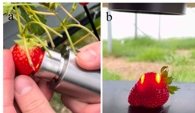
Fig. 2. (a) Illustration of contact measurement using MicroNIR in field. (b) Illustration of non-contact measurement with interaction prototype in field. This is a snapshot of interaction Distance 5 (8.5 mm), giving a distance between illumination lines of 17 mm.
