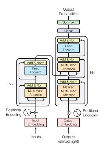
Figure 2.9: Building blocks of a Transformer [Vaswani et al. 2017]
