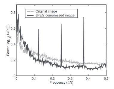
Figure 3.2: Power spectra of original and JPEG compressed image [Bovik and Wang 2006] that shows energy peaks on feature frequencies
