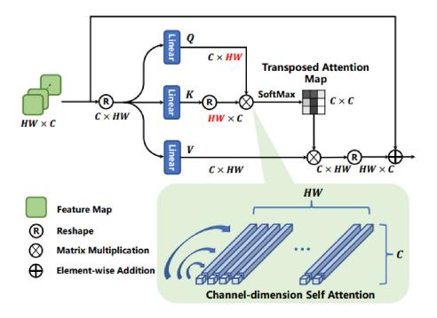
Figure 3.7: MANIQA transposed attention block [Yang et al. 2022]
