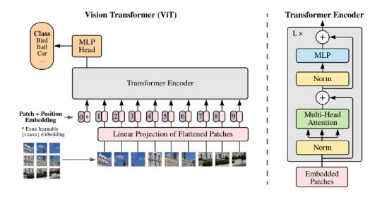
Figure 2.10: Vision Transformer [Dosovitskiy et al. 2021; Vaswani et al. 2017]
