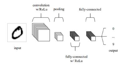
Figure 2.7: A simple 5-layer CNN architecture[O'Shea and Nash 2015]
