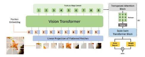
Figure 3.6: MANIQA network architecture [Yang et al. 2022]
