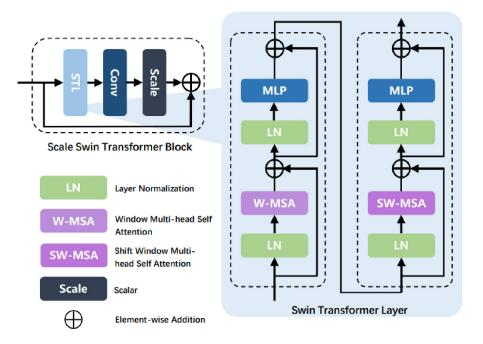
Figure 3.8: MANIQA scale swin transformer block [Yang et al. 2022]
