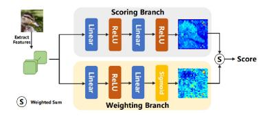
Figure 3.9: MANIQA dual branch patch-weighted quality prediction [Yang et al. 2022]
