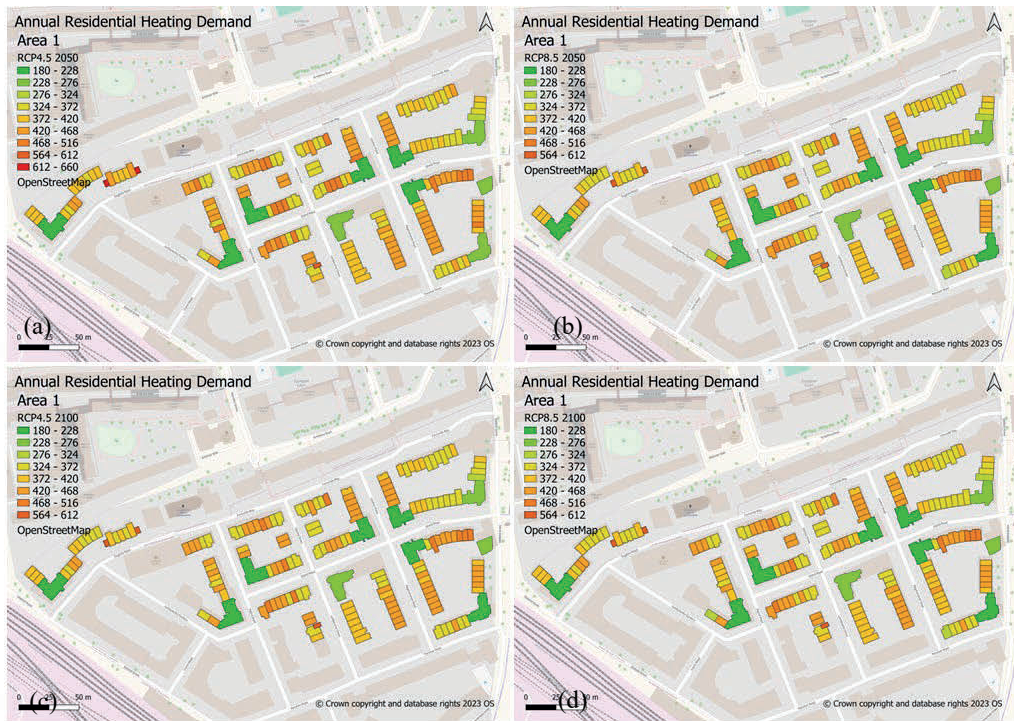
Fig. 4. Annual Residential Heat Demand for Future Climate Scenarios, Case Study Area 1. (a) Future Climate Scenario: RCP4.5, 2050. (b) Future Climate Scenario: RCP8.5, 2050. (c) Future Climate Scenario: RCP4.5, 2100. (d) Future Climate Scenario: RCP8.5, 2100.
