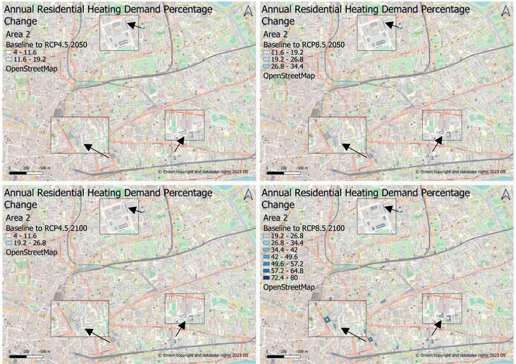
Fig. 8. Percentage Difference in Annual Residential Heat Demand from Present Climate to Future Climate Scenarios, Case Study Area 2.
