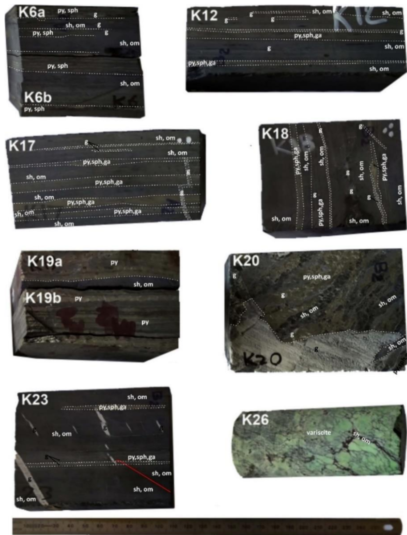
Fig. 2. Picture of eight (without K6b and K19a (see the main text)) mineralized dark clay rock samples from Zn-Pb Koushk mine. The samples have a relatively low porosity. Metallic minerals are found as interlayers within the shale background. All the samples have a layered structure besides the disseminated one. K20 and K26 differ from the others. White areas in K20 consist of gypsum. Green particles in K26 are Variscite. White dashed lines highlight the traces of shale and metallic layers. Shale (sh), organic matter (om), gypsum (g), pyrite (py), galena (ga), sphalerite (sph), and variscite are annotated.
