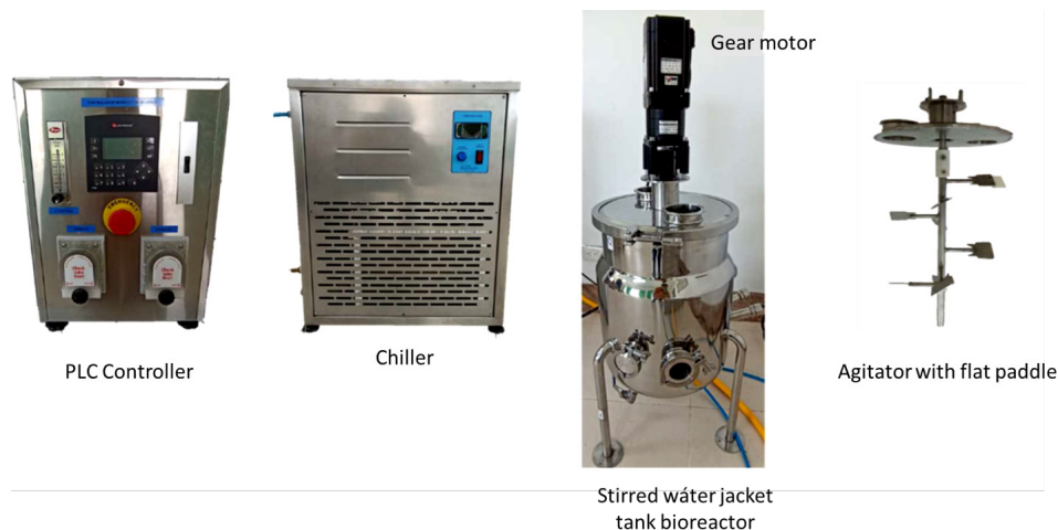
Figure 1. Design coffee stirred tank bioreactor equipment.
