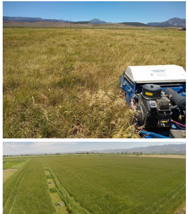
Figure 3. Using a Flail-Type Plot Forage Harvester (top) to Measure Yield in Each Treatment (bottom)
