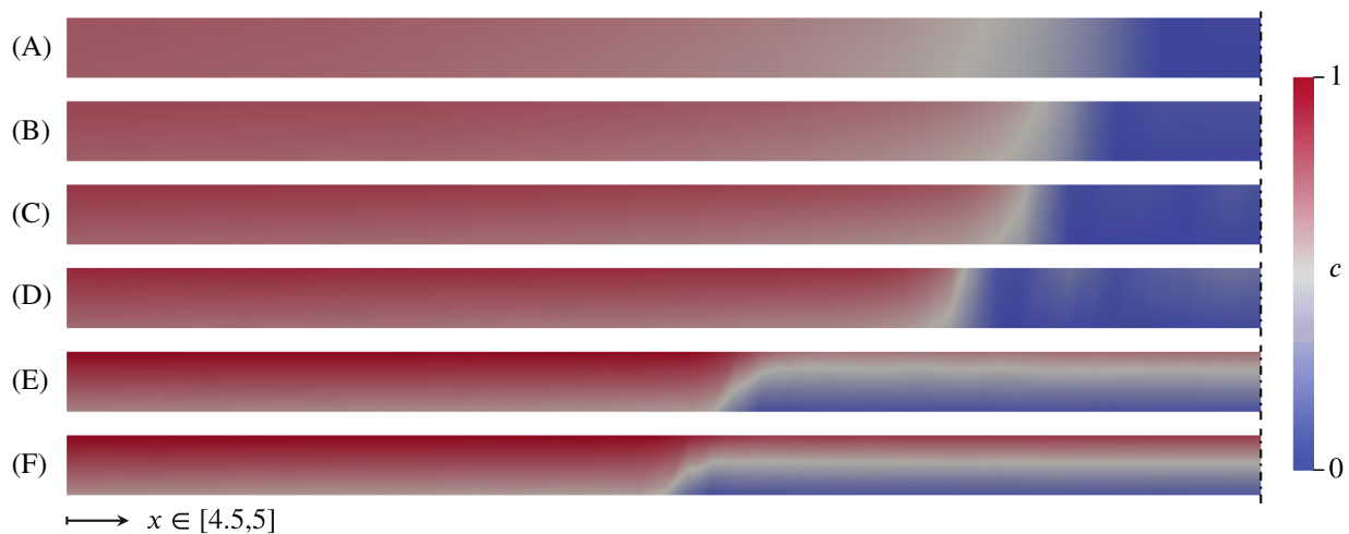
FIGURE 8 Simply supported beam, final phase-field as obtained with the mixed-dimensional model (side view). (A) l/t = 1/1 ; (B) l/t = 1/2 ; (C) l/t = 1/3 ; (D) l/t = 1/4 ; (E) l/t = 1/8 ; (F) l/t = 1/10
