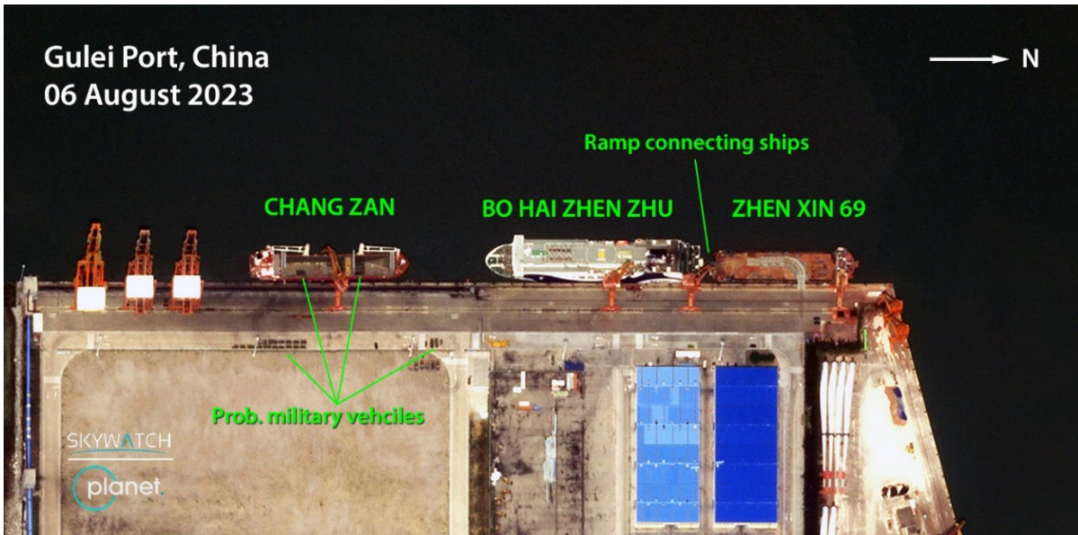
Figure 11. Variable Height Loading Ramp, Gulei, China, 06 August 2023 (© 2024 Planet) 17
