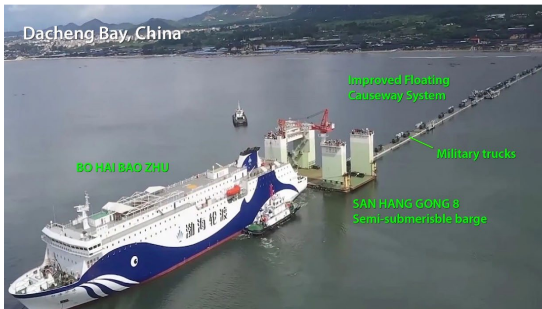
Figure 21. Floating Causeway, SAN HANG GONG 8, and RO-RO Ferry in JLSF Recruiting Video, 26 July 2023 37
