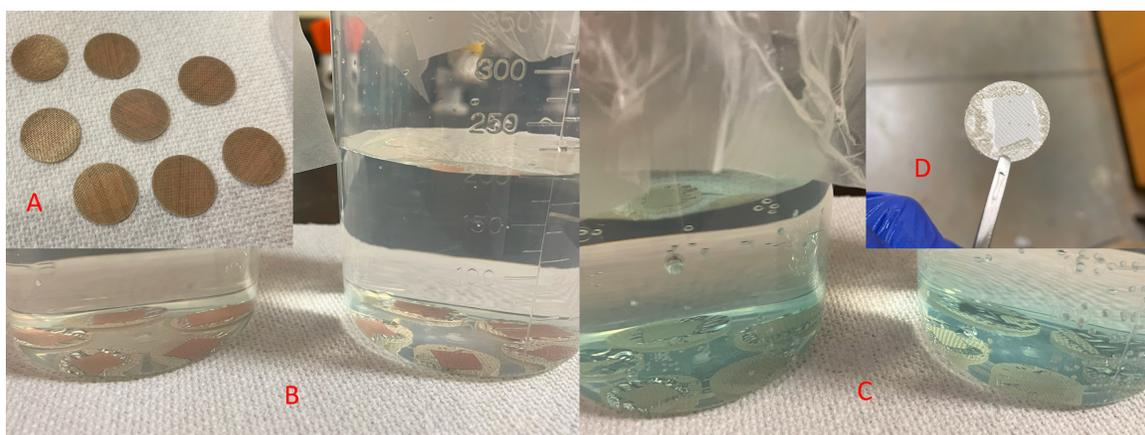
Figure 7.1: Process of CVD graphene transfer onto Nafion 211 membranes. A. CVD graphene on copper sheets hot-pressed onto single layers of Nafion 211 membranes. Teflon-reinforced fiberglass sheets were placed from either side of it prior to hot-press. B. Copper—graphene—Nafion composites were immersed in 0.3 M APS solution. C. and D. Post-etched graphene-deposited membranes.
