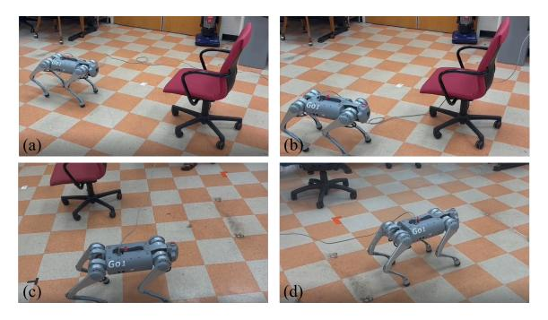
Figure 4.9: Feedback Density Planner on Go1 Hardware without a motion capture system. Extra enlargement of the obstacle set was done to account for state estimation drifts. The following figure shows the Unitree Go1 at a) start, b) beginning to avoid  $X_u$ , c) after avoiding  $X_u$ , and d) goal
