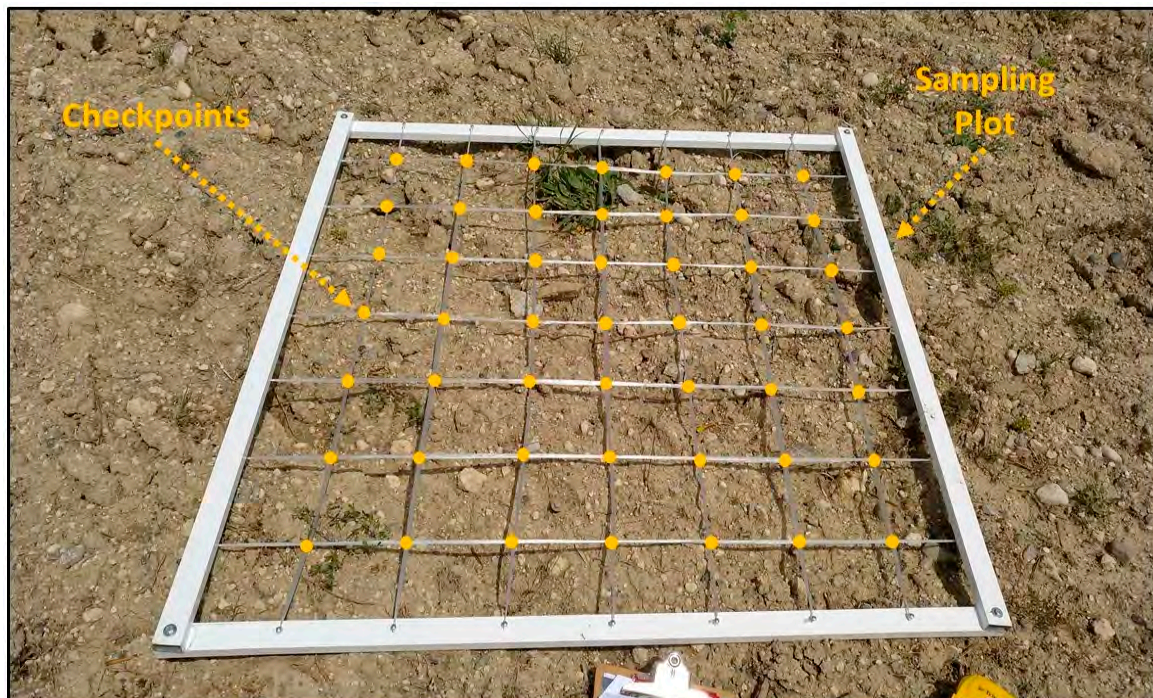
Figure 4. Quadrant-based method for quantifying VGC.
