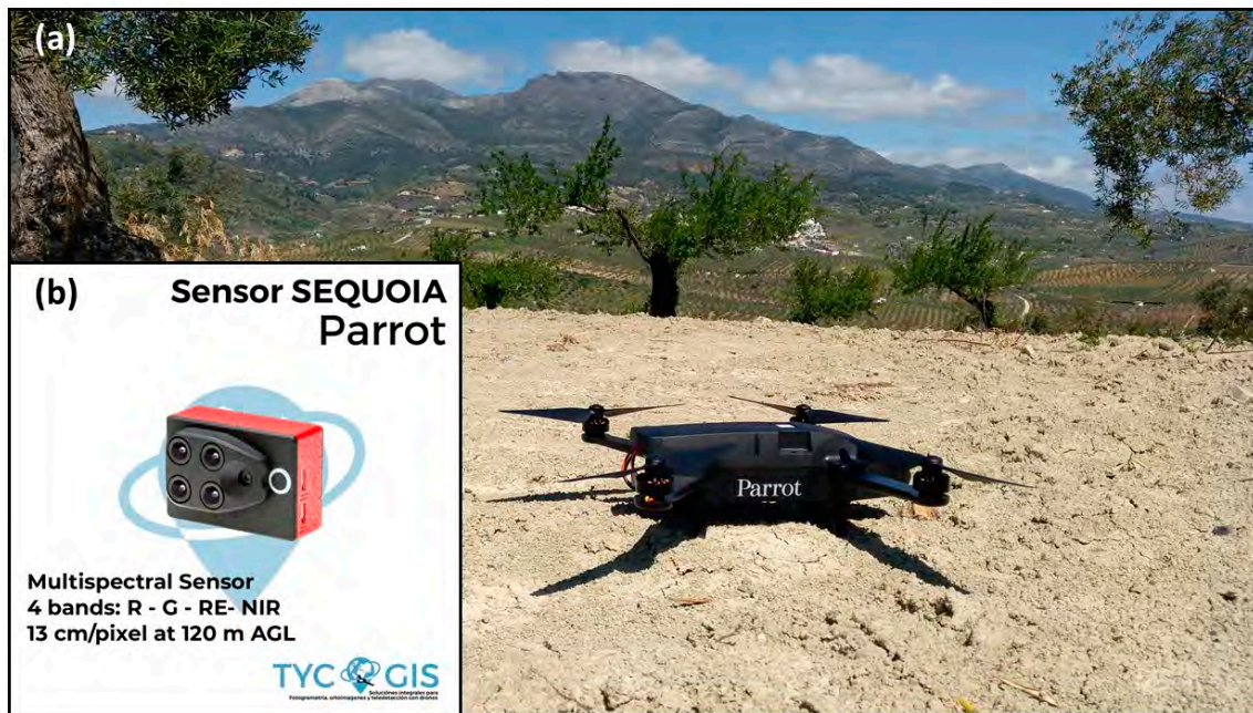
Figure 3. UAV quadcopter (a) and multispectral sensor (b).
