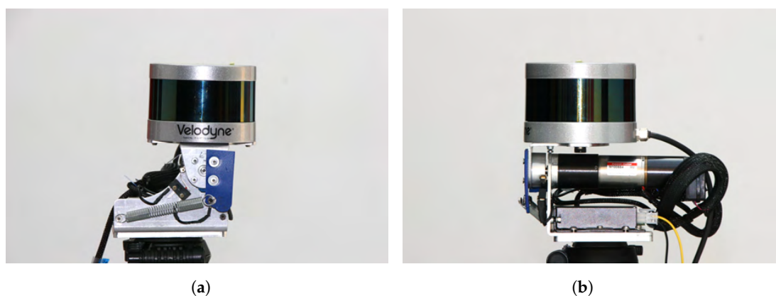
Figure 8. Views of the Velomotion-16 RMBL sensor: (a) side; and (b) front.
