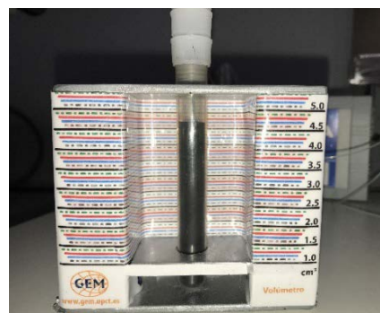
Figure 3: Volumeter designed with a parallax error control ( 4.7 \pm 0.1 \text{ cm}^3 readable)
