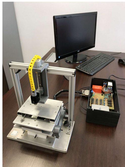
Fig. 14 Micro-machining tool prototype. Two-dimensional control system
