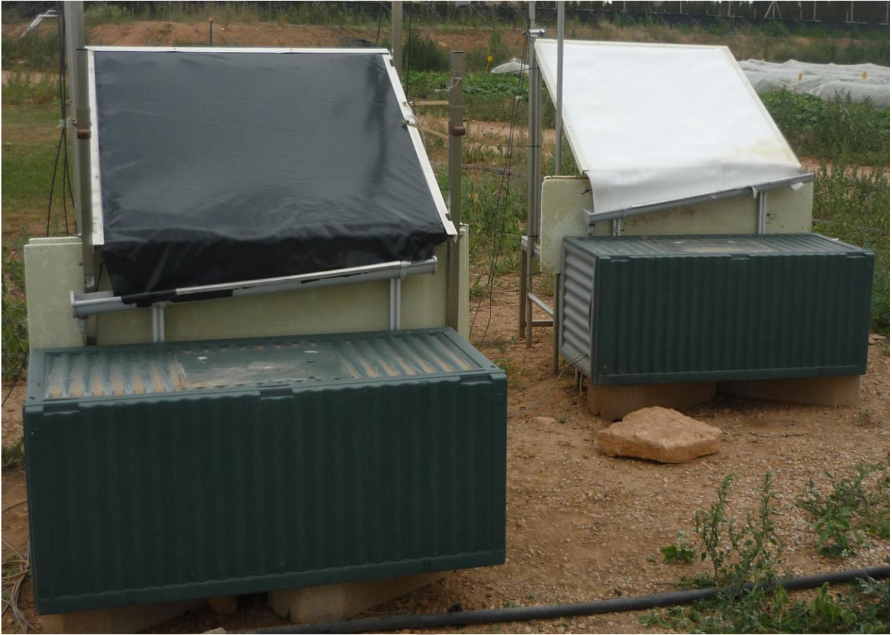
Figure 1. View of the two radiative dew condensers with the black PE foil (BF) and the white standard foil (WSF) fitted to the 30° tilted flat pans.
