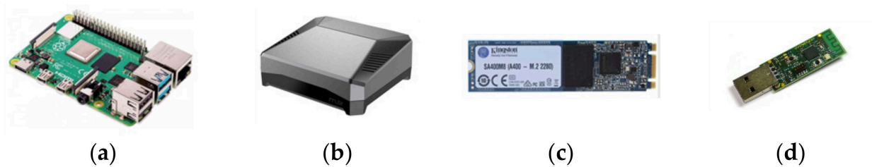
Figure 4. (a) Raspberry Pi, (b) Raspberry Pi Aluminum Case, (c) SSD Memory Disk, (d) USB Dongle cc2531.
