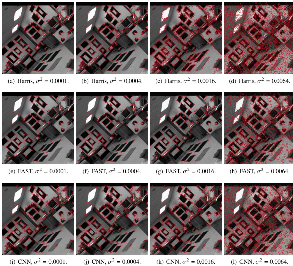
Fig. 11. Localization of pixels with multiple orientations using the Harris corner detector (first row), FAST (second row) and a CNN (third row). The 256 \times 256 gray-level images “Lab” has been degraded with additive Gaussian with variances \sigma^2 = 0.0001 (first column), \sigma^2 = 0.0004 (second column), \sigma^2 = 0.0016 (third column) and \sigma^2 = 0.0064 (fourth column).
