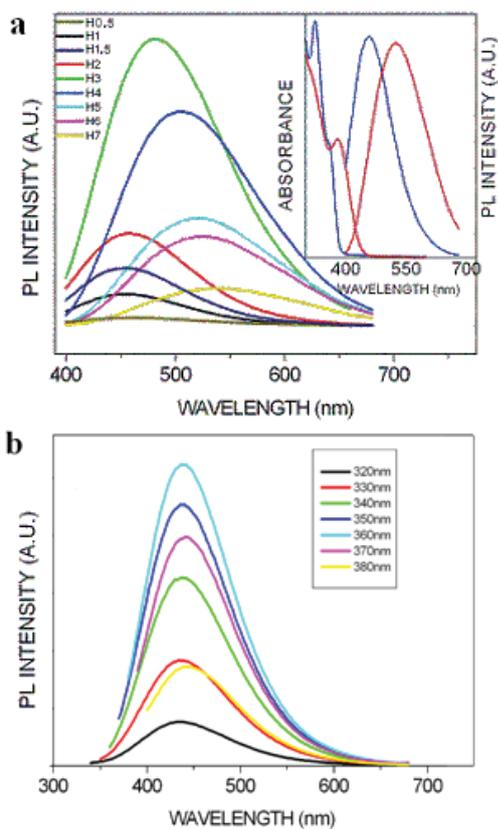
**Figure 4.** PL emission spectra for GSH-CdS QDs solutions obtained from the reaction flask over the course of the entire reaction process using an excitation wavelength of 380 nm (a); and PL emission spectra for the H1 sample obtained for different excitation wavelengths (b).
