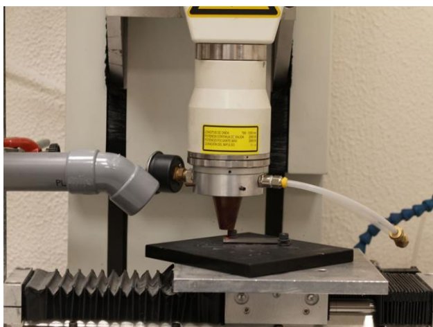
Fig. 1 High Power Diode Laser (HPDL) head, mobile XY table and shielding gas system
