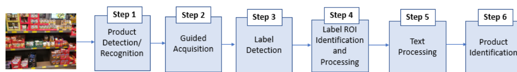
Figure 3. Conceptual pipeline of assisted retail product label analysis.
