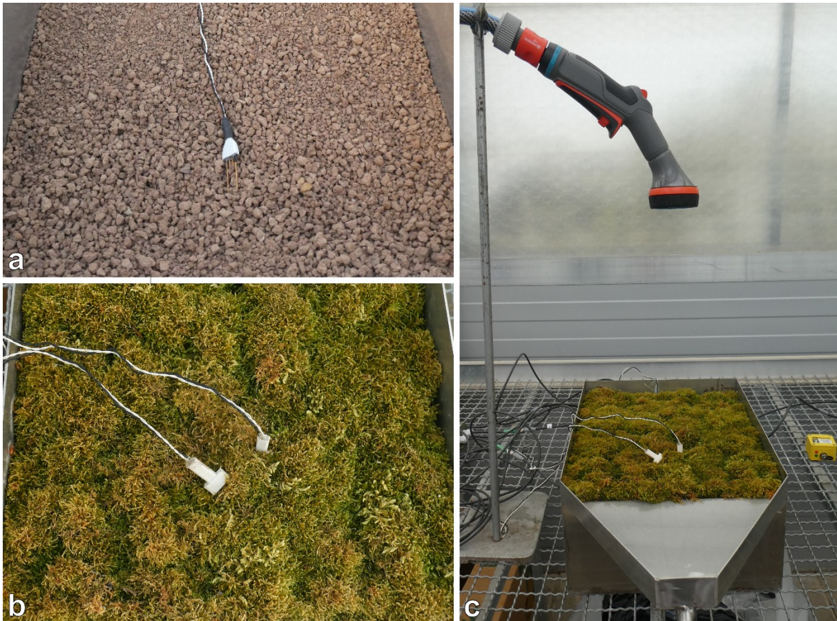
Figure 7: Overview of the greenhouse experiment setup. (a) Biocrust wetness probe (BWP) in 3 cm substrate depth before refilling with another 3 cm substrate layer. (b) BWP at the substrate surface and in the moss cover. (c) Experimental setup with moss-covered substrate inside the infiltration box and sprayer.
