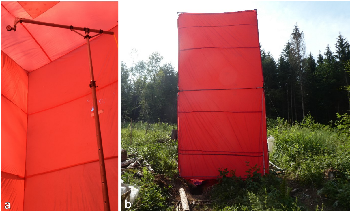
Figure 5: The Tübingen rainfall simulator with protective tent. (a) The Tübingen rainfall simulator inside the tent. (b) The protective tent in the field (2 x 2 m ground area, 4 m height).
