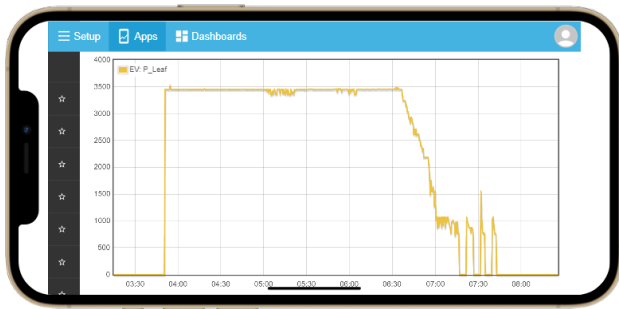
Fig. 11. A charging cycle of a Nissan Leaf to 100%
