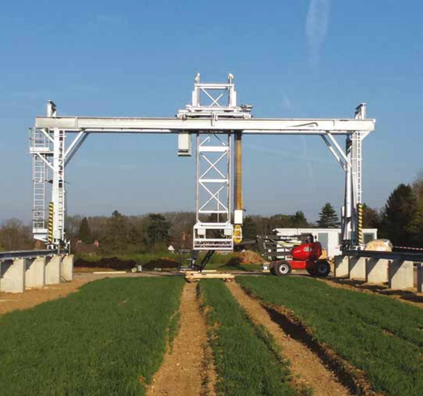
Field scanner at Rothamsted Research – the world's first fully automated field facility for measuring crop growth and health. Source: Achim Dobermann
