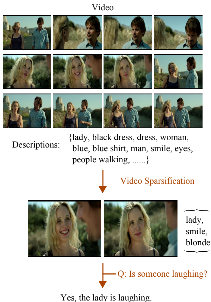
Figure 4.2: We study the Sparsified VideoQA problem, where we learn to sparsify the original long video into very few inputs for QA. We design a video sparsification process to deal with video of multiple modalities (frames, word and phrase descriptions, etc).
