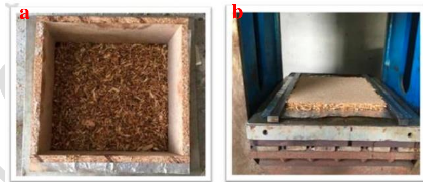
Figure 1: Preparation of particle mat (a) and board consolidation by pressing the mat using hydraulic press (b).
