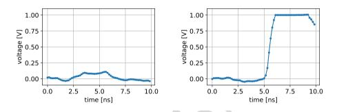
Figure 4. Examples of noisy (left) and saturated (right) events acquired using the diamond sensor
