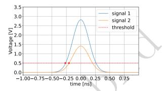
Figure 2. Time walk error illustrated as a difference in the threshold crossing times between two signals with the same shapes but different amplitudes
