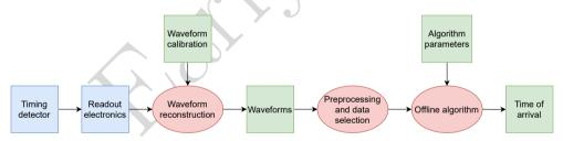
Figure 1. Data flow diagram for the analysis of the timing data (blue: electronics, green: data, red: digital algorithm). Multiple algorithms can be used to retrieve the time of arrival from the waveform data. In this research we focus on digital algorithms working in the offline mode.
