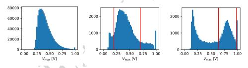
Figure 5. Maximum voltage histograms for MCP (left) and two selected diamond detectors (middle and right). The red lines on the histograms of the diamond detectors indicate the minimum and maximum amplitude cuts. It is important to note that the histograms look different for each detector, and therefore, it was necessary to find the amplitude cut values separately for each of them.
