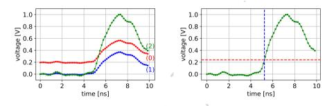
Figure 7. Depiction of the CFD algorithm. Left: (0) before normalisation, (1) baseline subtraction, (2) division by maximum. Right: when the normalisation is done, the timestamp can be found using the fixed threshold algorithm. The threshold chosen for this example is arbitrary.
