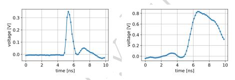
Figure 3. Example waveforms from the MCP (left) and a diamond detector (right).
