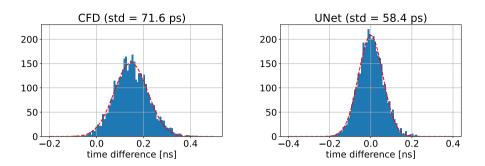
Figure 11. Difference histograms for the CFD and our best-performing, UNet-based model
