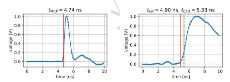
Figure 6. Example from the final dataset. Left: waveform from MCP.  $t_{\text{MCP}}$  (red line) is computed using the CFD. Right: waveform from a diamond detector.  $t_{\text{ref}}$  (red line) is the neural network's reference time computed using the CFD for the MCP waveform. The green dashed line represents the time computed using the CFD with the waveform from the diamond detector ( $t_{\text{CFD}}$ ). It is not included in the dataset and is shown only for visualisation purposes.
