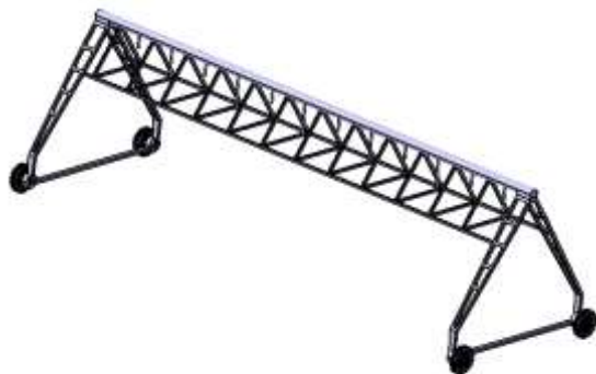
Fig. 1. Solid works of hanger irrigation system
