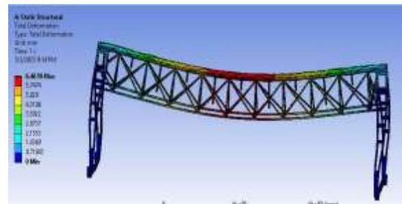
Fig. 24 The total deformation is observed to be 6.4659 mm
