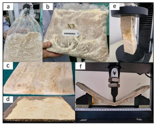
**Figure 1.** Bio-composite production and testing. a) Ganoderma sp. spawn, b) Fully colonized Ganoderma sp., grown in Albizia sawdust as the lignocellulosic substrate c) Bio-composite grown in a 30 x 30 cm cast and dried, d) Bio-composite after hot-pressed, e) Compressive strength measurement, f) Flexural strength measurement with 3-point bending test.
