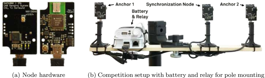
Figure 4: Hardware used in the competition by the ATLAS team. Note the orientation of the anchor node antennas. The antenna of the nodes is mounted upwards, with the flat side facing the competition.
