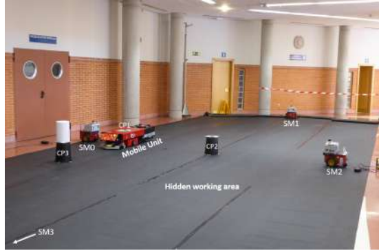
Figure 10: Working area covered by sensor modules (SMs), calibration points (CPs) are also included (ALCOR team).
