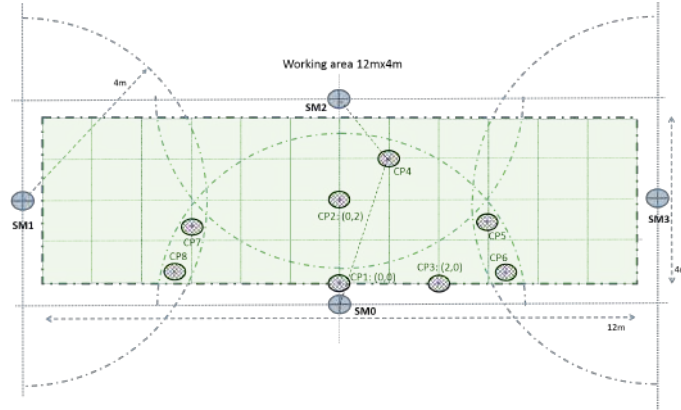
Figure 11: Sensor modules and calibration points involved in the calibration procedure.
