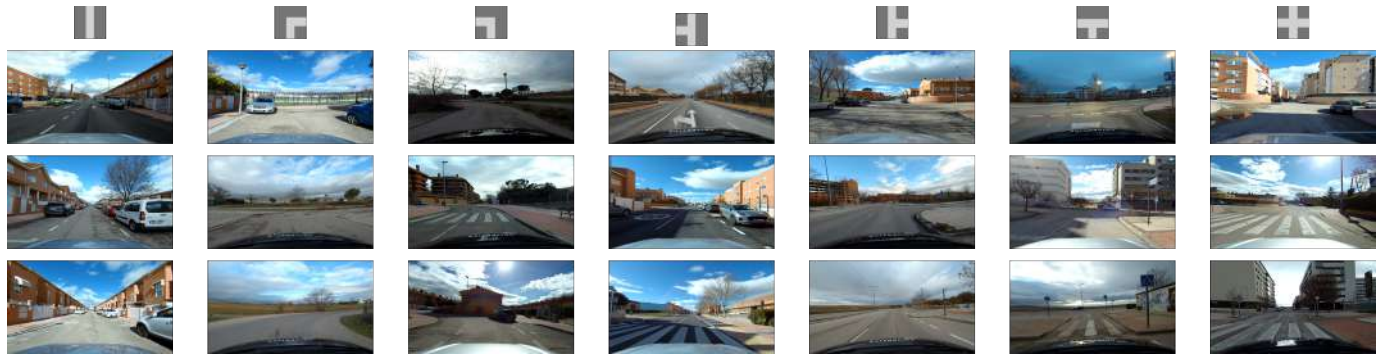
Figure 5. Each column shows three examples of the seven configuration geometries that were used in this work (with the so-called canonical images shown in the upper part of each column). The RGB examples come from our recorded dataset. We recorded the images at different times of the day using a different camera setup for more than 3:30 h of recording time, including more than 500 intersections.
