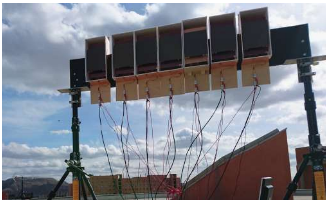
Fig. 23. Designed array integrated in IDEPAR demonstrator in the radar scenario.
