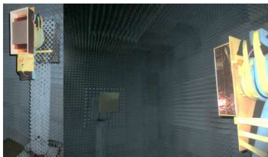
Fig. 15. Prototype antenna characterization in anechoic chamber.
