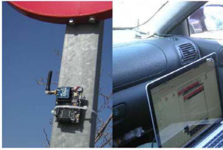
Fig. 7. Left: Waspnote transmitter installed on a signal. Right: Waspnote receiver in the test-car.
