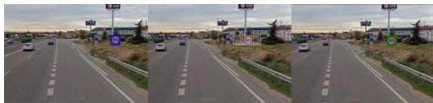
Fig. 4. (Left) Left image and bounding box of the detected speed sign. (Middle) Search space along the epipolar line corresponding to the upper-left part of the bounding box on right image. (Right) Final match on right image.
