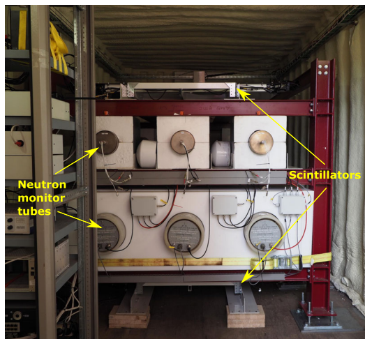
Figure 2: ORCA setup, including the two MITO devices at the top and bottom and NEMO in between.
