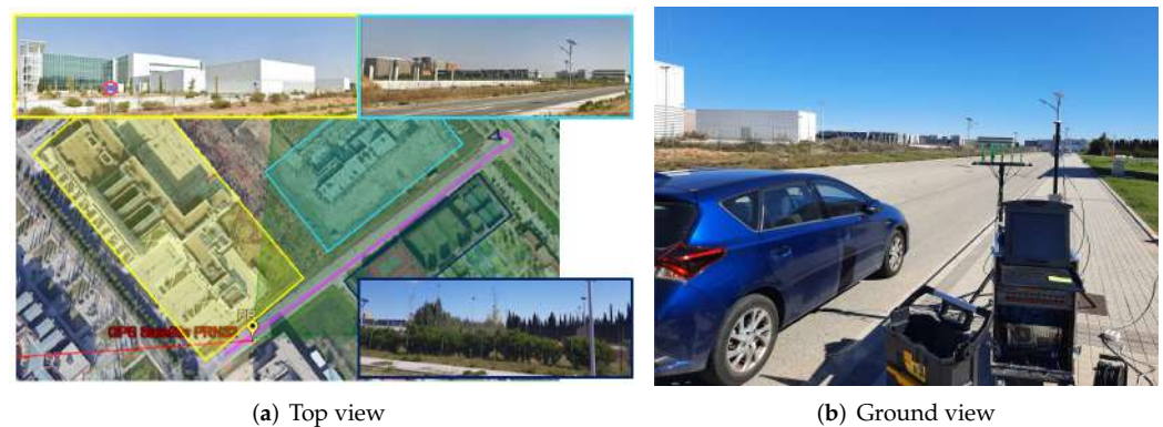
Figure 10. Trials radar scenario: (a) top view with PR location, satellite direction (PRN32), area of interest (green area), cooperative target trajectory from GPS data (purple line), buildings and sport facilities details are shown in pictures with their associated area; (b) ground view of the AoI, cooperative vehicle and PR receiver deployment.
