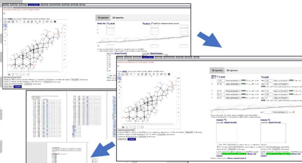
FIGURE 3 Outputs of the NMRdata javatools viewer. Left upper: Structure and shift list entered. Right: Automatic assignment done and checked. Left lower: The NMRdata file exported. The list of shifts has been shortened.
