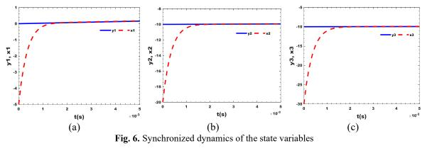
Fig. 6 (a), (b) and (c) depicts the synchronization of the dynamics of the master ad slave system. it can be seen that the trajectories coupled in less than 0.002s. these are relatively fast. The stabilized dynamics of the synchronization error functions and the finite time control law are shown in Fig. 7 and Fig. 8 respectively.
