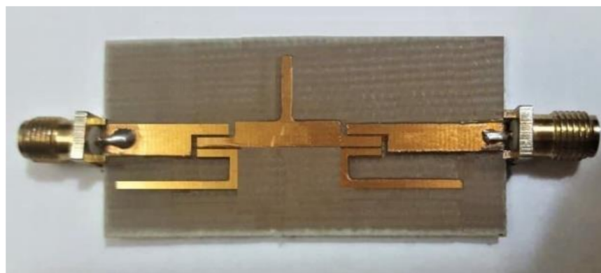
Figure 10. The prototype of the proposed microwave filter.
