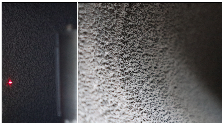
Fig. 4. Detail of the particle layer: laser light from the distance sensor (left), and macroscopic structure (right).
