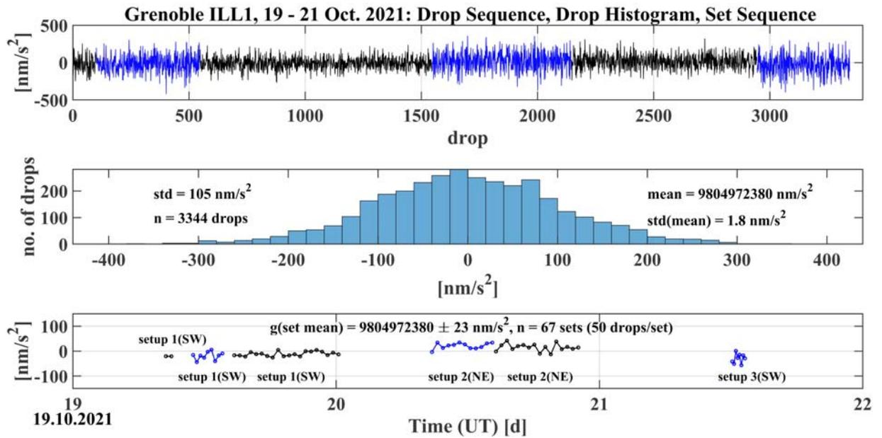
**Figure 1:** Statistical compilation of the station determination with the Hannover FG5X-220 absolute gravimeter at ILL Grenoble in October 2021
