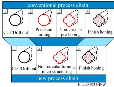
Fig. 2. Conventional and new process chain.
