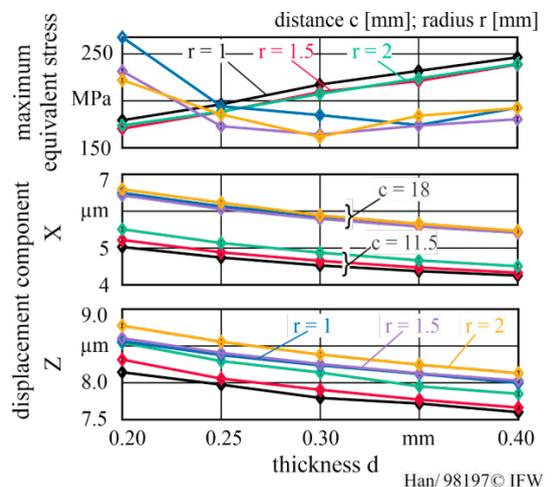
Fig. 7. Displacement of the cutting edge due to process forces.
