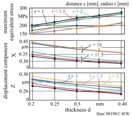
Fig. 6. Equivalent stresses due to the displacement  $\Delta u$  of the piezo actuator.
