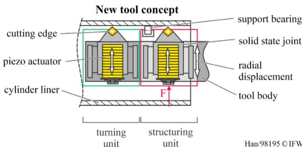
Fig. 4. Actuator concept of the hybrid tool.
