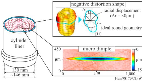
Fig. 1. Approaches to reduce the friction in the piston-cylinder system.
