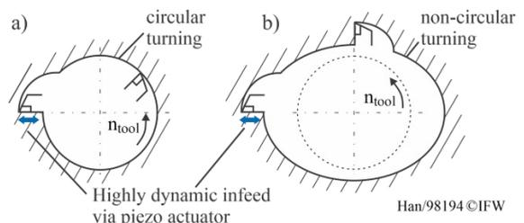
Fig. 3. Microstructuring into a) circular turned cylinder liner, b) non-circular turned cylinder liner.
