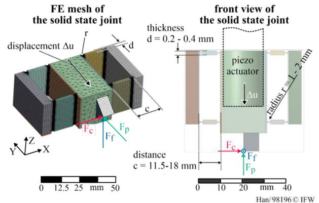
Fig. 5. Solid state joint.
