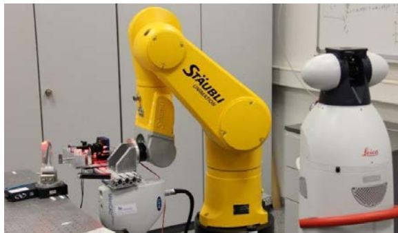
Fig. 5 Robot guided microscale fringe projection system
